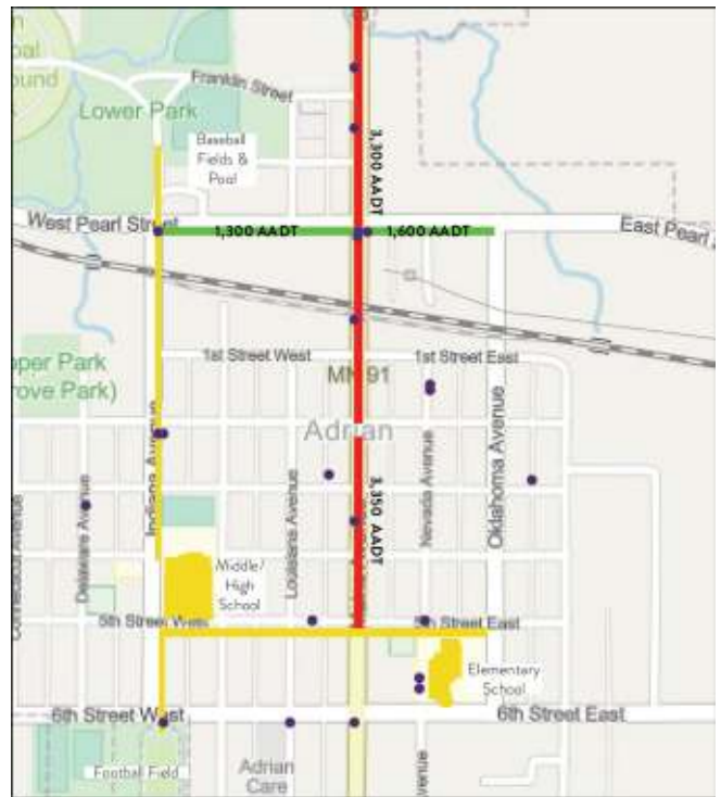
Traffic volumes, school destinations and crash data for the City of Adrian
